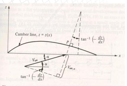
Figure 4.23 Determination of the component of freestream velocity normal to the camber line.
